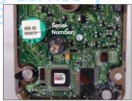
Figure 2 - Serial # on Label on Capacitor
